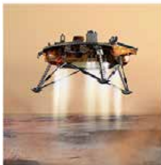
Figure 7.12 The landing craft suspension can be represented as a damped spring-mass system. (credit “lander”: NASA)
